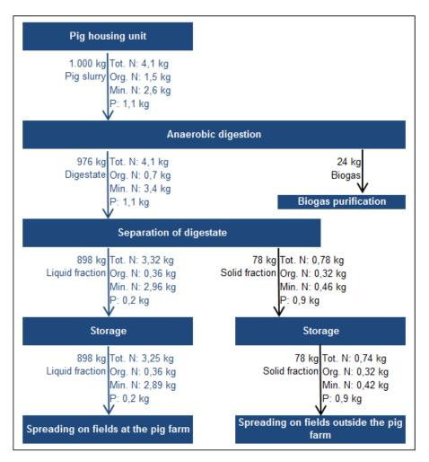
Figure 1. Simplified flow chart for optimal pig manure handling. Pig slurry is treated in a biogas plant, the digestate is separated and only the liquid fraction is applied to the fields of the pig farm.
