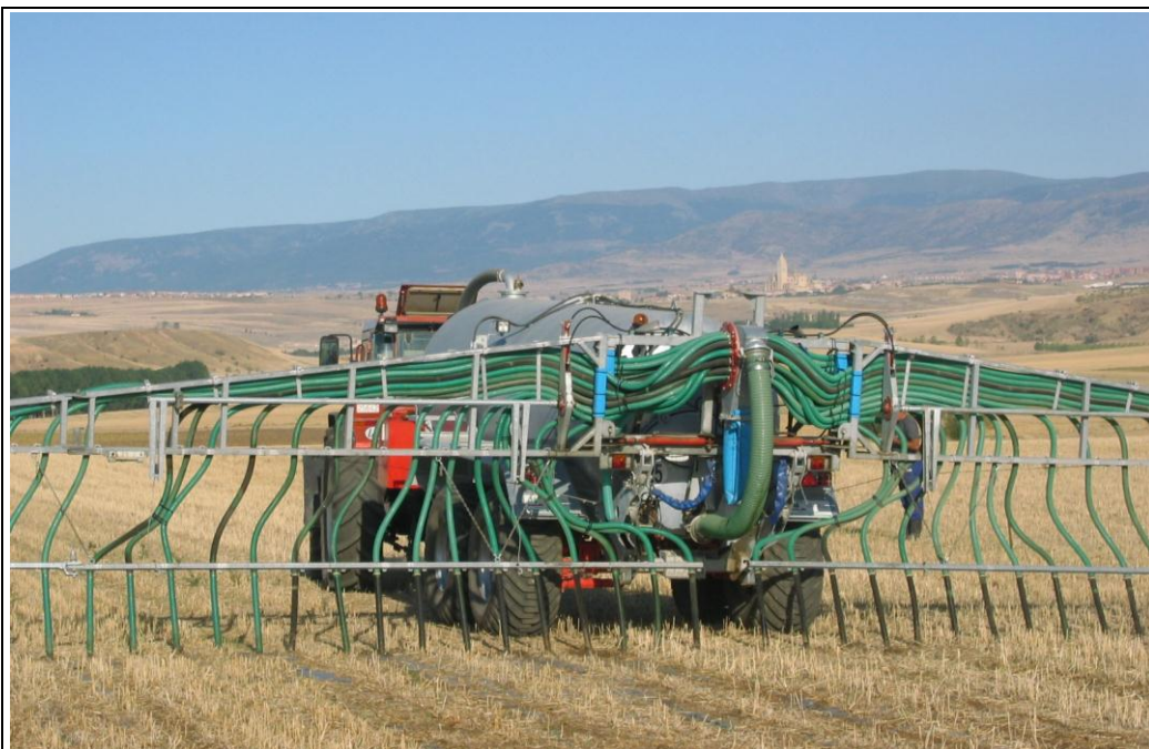
Figure 2.44: Example of a band spreader fitted with rotary distributor to improve lateral distribution
