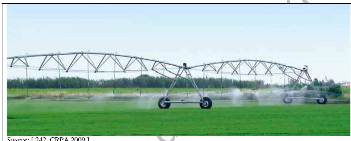
Figure 4.96: Irrigation boom fitted with hanging nozzles to spray slurry-mixed water close to the soil surface
