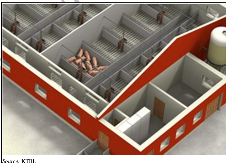
Figure 2.22: Scheme and layout of fully slatted floored pens in a fattening pig house
