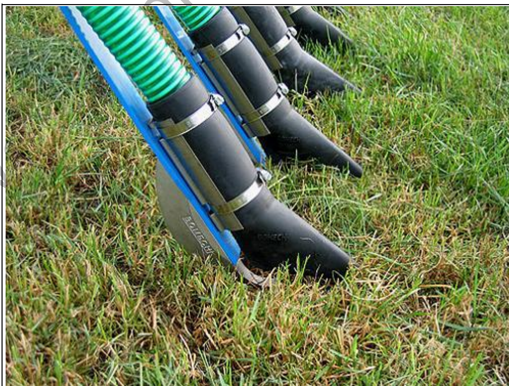
Figure 2.45: Example of a trailing shoe spreader
