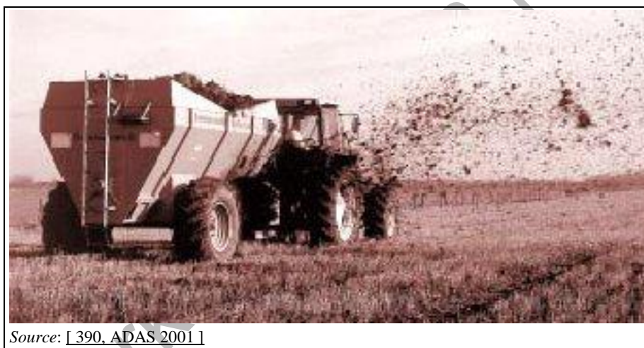
Figure 2.49: Example of a dual-purpose spreader
