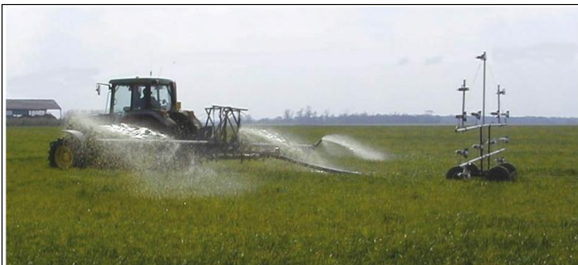
Figure 2.43: Side view of a horizontal boom with splash plate for slurry application
