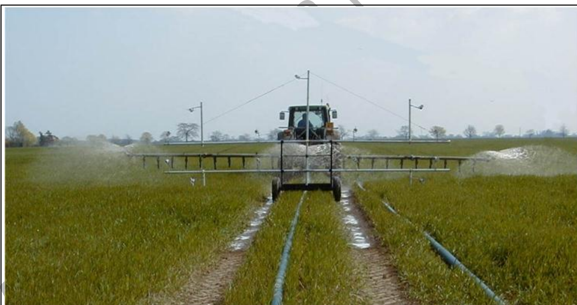
Figure 2.42: Rear view of a horizontal boom with splash plate for slurry application
