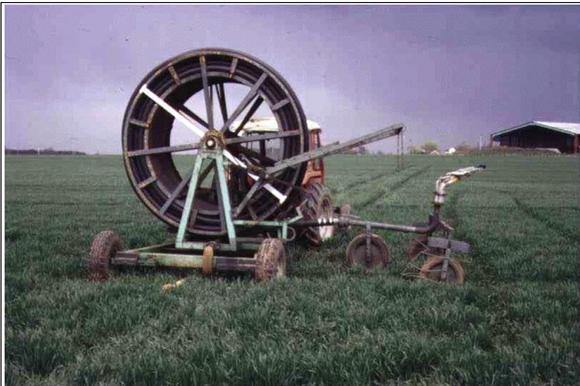
Figure 2.39: Example of a raingun
