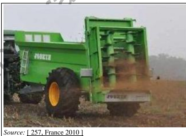
Figure 2.50: Vertical drum manure spreader
