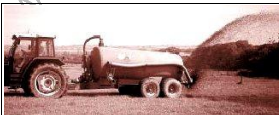
Figure 2.38: Example of a broadcast spreader with a splash plate
